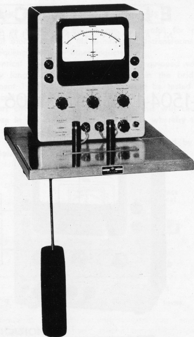
Fig. 3. Deviation Bridge mounted on the Test Jig Type 3902 for production line testing.
